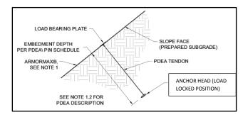
Figure 4: Type B1 Anchor Detail
