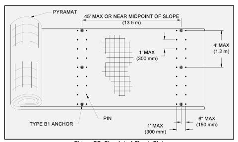
Figure 23: Simulated Check Slot
