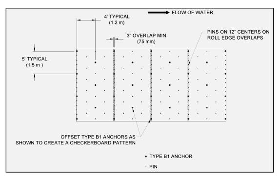
Figure 22: Example Anchor Pattern - 0.5 Anchors/ Yd2
