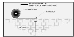
Figure 17: Initial Channel (IC) Trench Complete
