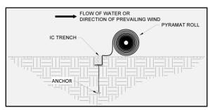
Figure 14: Initial Channel (IC) Trench Placement
