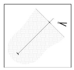
Figure 11: Trim Extra Cable Flush to Plate
