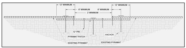
Figure 28: ARMORMAX® Patch Cross Section
