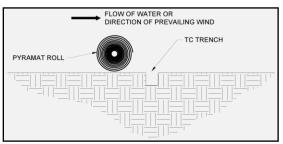
Figure 18: Terminal Channel (TC) Trench Alignment
