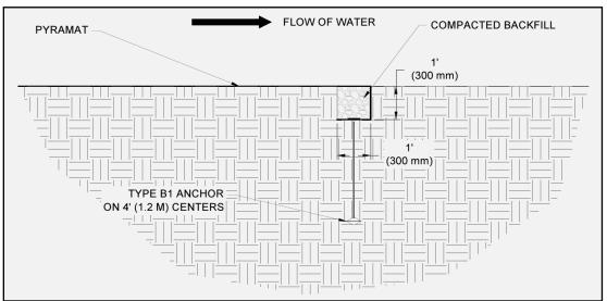
Figure 1: Initial Channel (IC) Trench
