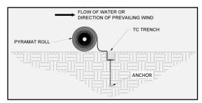
Figure 19: Terminal Channel (TC) Trench
