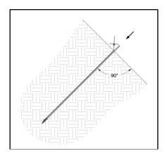
Figure 7: Drive Steel to Drive the Type B1 Anchor into the Ground
