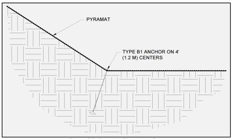
Figure 25: Break in Slope Interface
