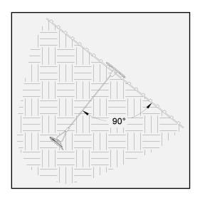
Figure 12: Complete Type B1 Anchor Installation
