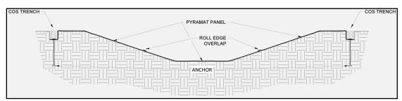
Figure 26: Crest of Slope (COS) Placement
