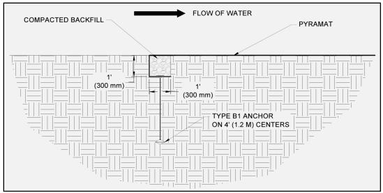
Figure 3: Terminal Channel (TC) Trench
