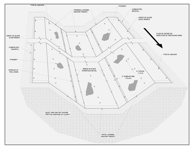
Figure 27: Completed Channel Isometric View
