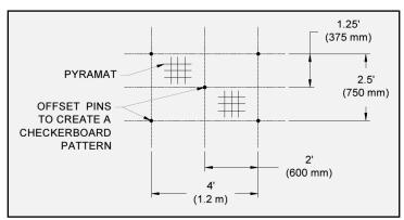
Figure 21: Example Pin Pattern
